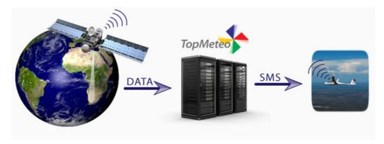
The above shown picture displays the schematic from the satellite image via the TopMeteo.eu server to the cell phone receiving the *FlySat-Message* in flight.
